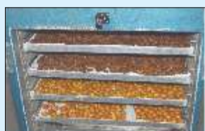
Fig. Drying of dates in air circulating tray drier
